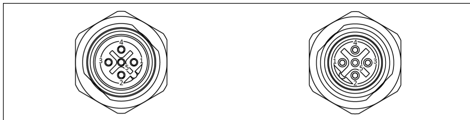
PIN allocation of socket and plug for Profibus oder CAN bus
